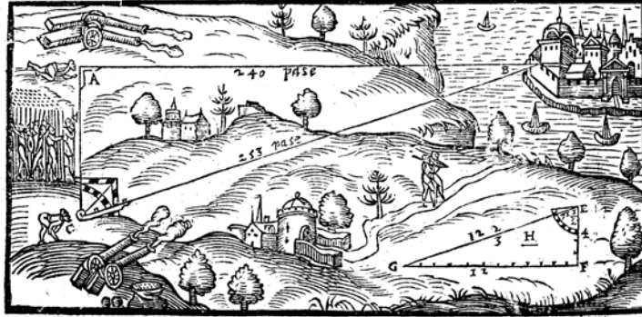
Fig. 4.24: Scene with an auxiliary triangle from Digges (1571, Sig.G3 v )
